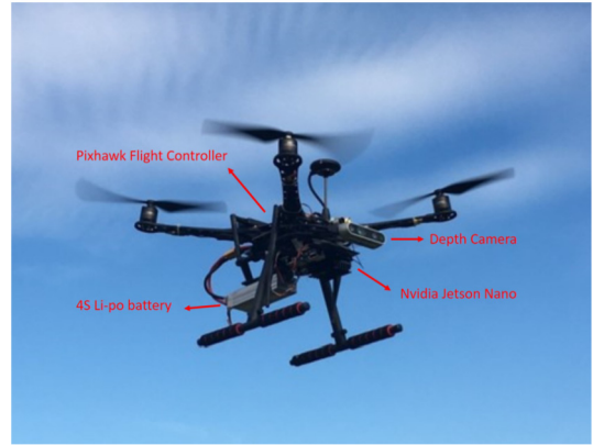
Fig. 12. Self-assembled quadrotor platform used for real flight test.
